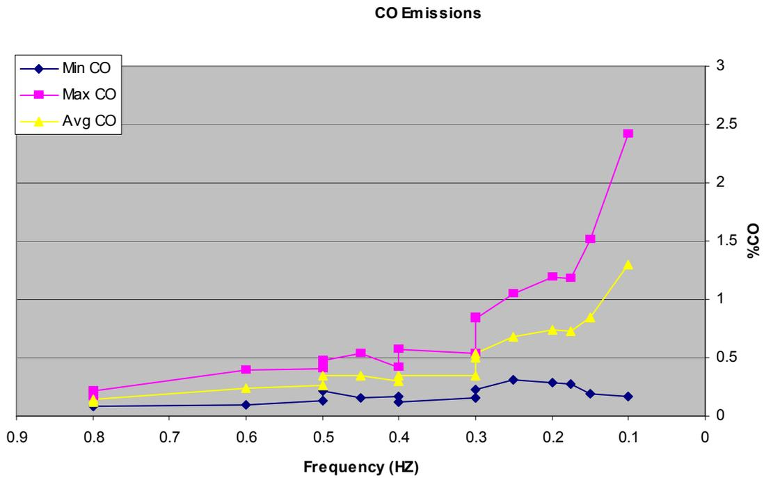
Figure 1 shows a clear rise at 0.3Hz it is clear that at that point the catalytic converter stops converting CO.
