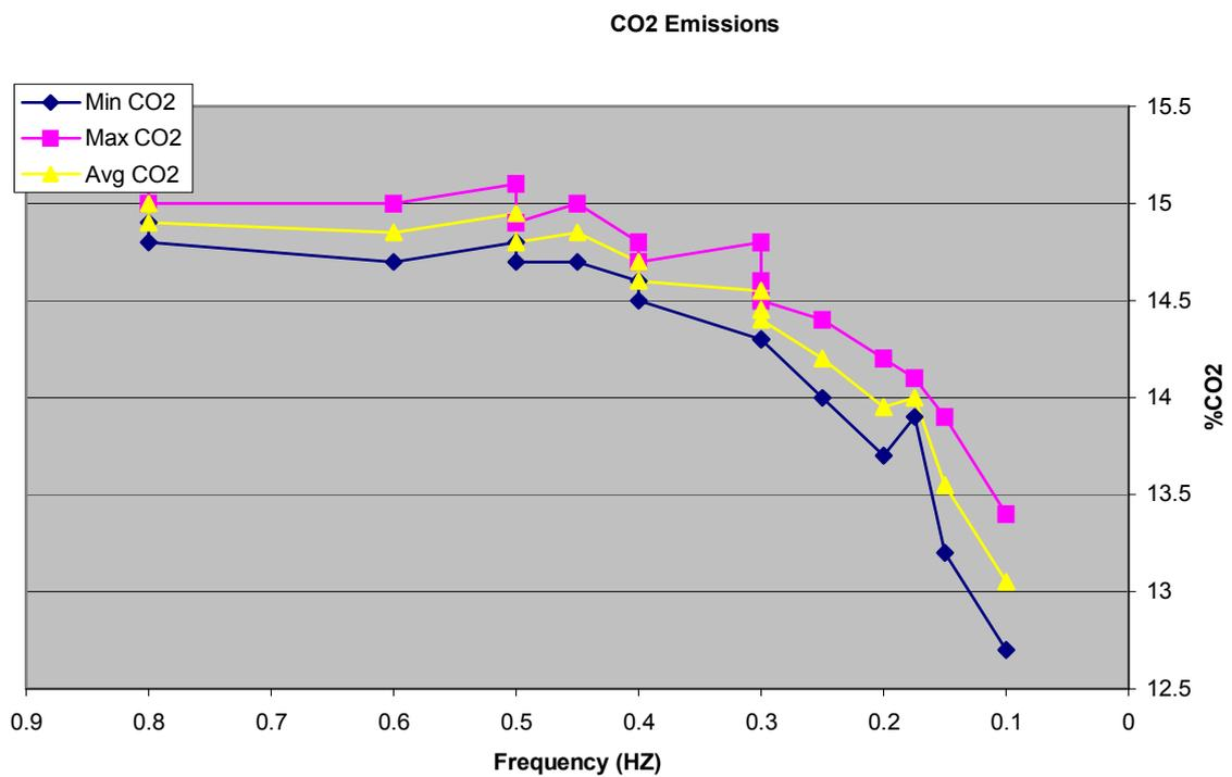
*In figure 3 it can be seen that the CO<sub>2</sub> clearly starts decreasing at 0.5Hz, showing that the operation of the catalytic converter starts deteriorating at this point.*
