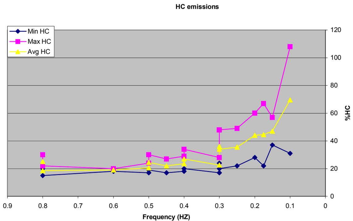
Figure 2 shows a clear increase at 0.3Hz also showing that at that point the catalytic converter has stopped converting HC.
